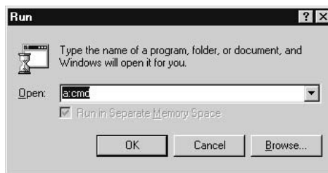
Figure 5-5. Running a trusted version of cmd.exe
