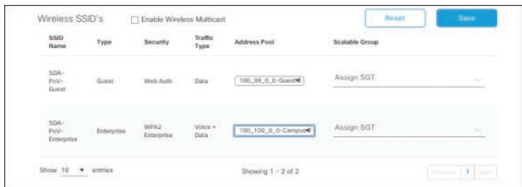
Figure 4-24 IP Pool to Wireless SSID Assignment
