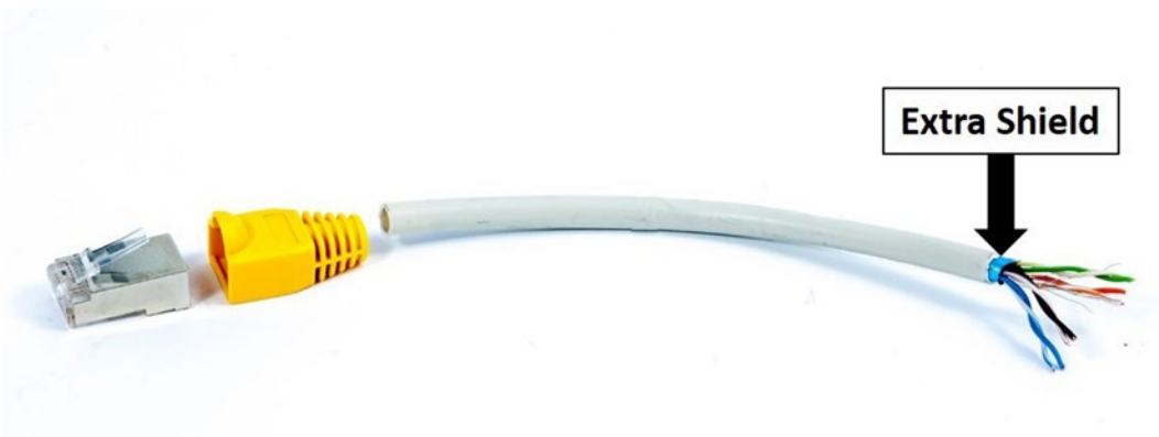
Figure 2-3. Shielded twisted pair cable (Photo copyright Sergio Bertino | Dreamstime.com. )
