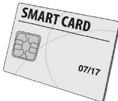
FIGURE 10.1 A smartcard's ISO 7816 interface
