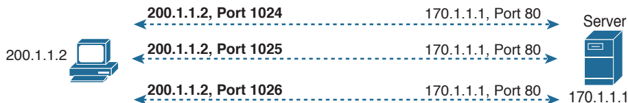
Figure 27-7 Three TCP Connections from One PC
