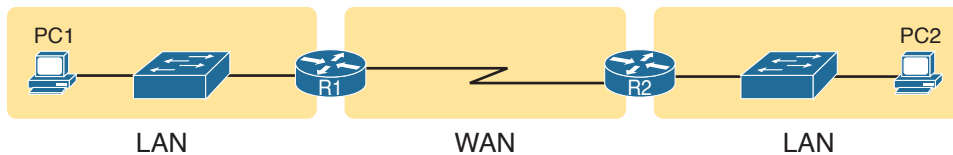
Figure 3-1 Small Enterprise Network with One Leased Line
