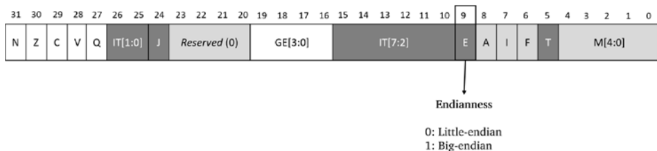
Figure 4.15: Endianness bit location in the CPSR
