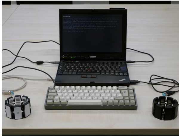
Fig. 2. The setup for the data collection showing the two Myo armbands in the front.
