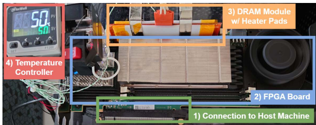
Figure 4: Our DDR4 DRAM testing infrastructure.
