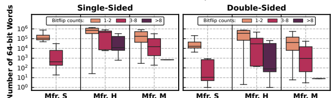
Figure 21: Number of 64-bit words with different bitflip counts for single-sided (left) and double-sided (right) RowPress.
