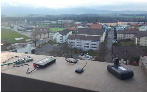
Figure 18: Picture of the measurement setup: Raspberry Pi 4, HackRF One, Iridium antenna, Iridium GO!
