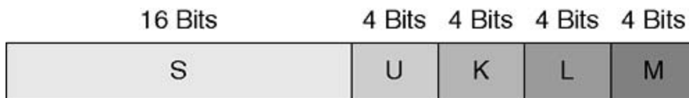
Figure 8-9. SONET/SDH Label Format
