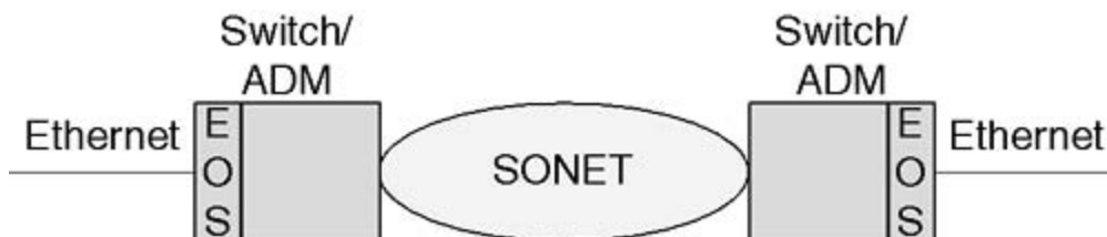
Figure 2-4. EOS and Switching Functions Inside the ADM
