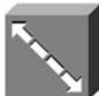
ISDN/Frame Relay Switch
