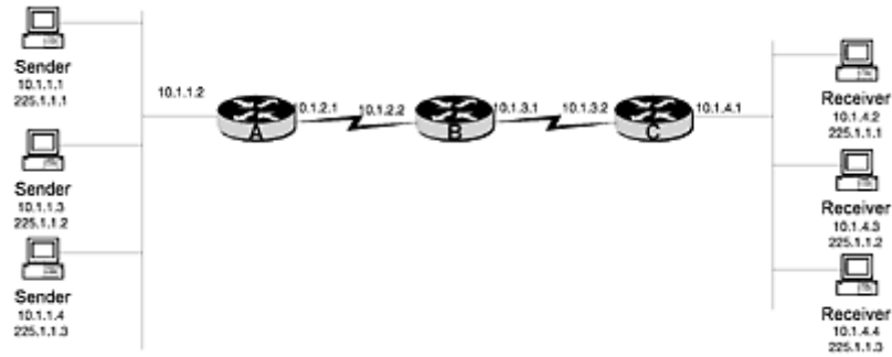
Figure 10-37 Example of static RSVP reservations
