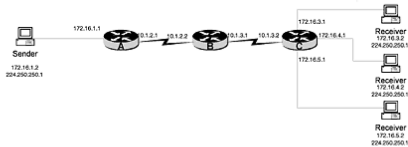
Figure 10-39 RSVP scenario with multiple receivers and a single source
