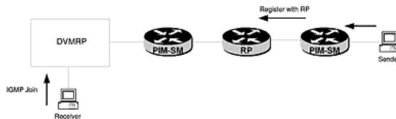
Figure 8-8 When the border router and RP are different, multicast traffic cannot be forwarded to the DVMRP receiver.
