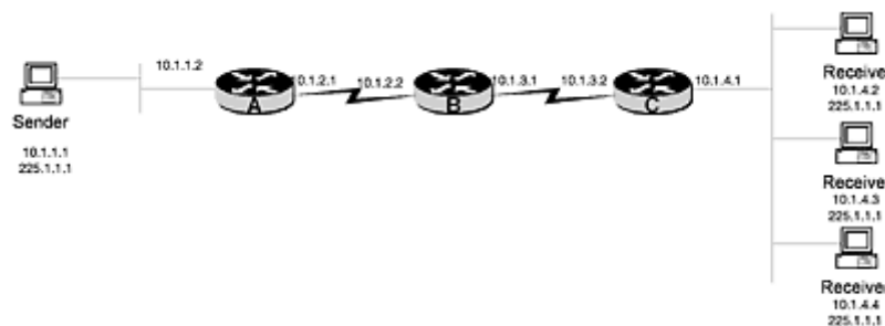
Figure 10-35 Allow only sender 10.1.4.2 to request a reservation
