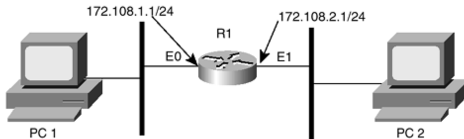
Figure 2-1. Routing IP with Directly Connected Networks
