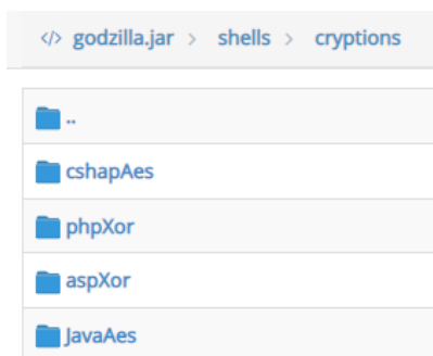
Figure 8. Cryptographic functions found in the source code of Godzilla Webshell. In case the victim's machine runs CSharp or Java the AES algorithm is used; else a simple XOR algorithm is implemented.
