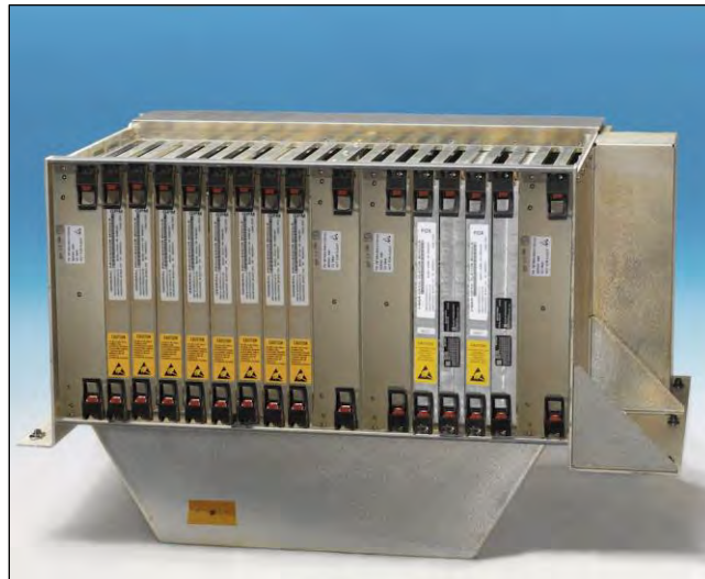
Figure 3. Boeing 787 CCR Cabinet 17
