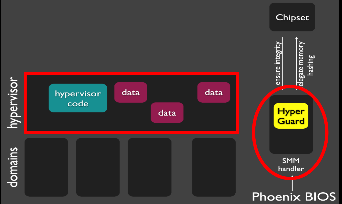
Figure 1: HyperSentry's architecture (Trusted components are shown in gray.)
