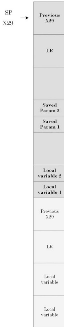
Figure 11-1. Stack memory layout for the function with two arguments and two local variables
