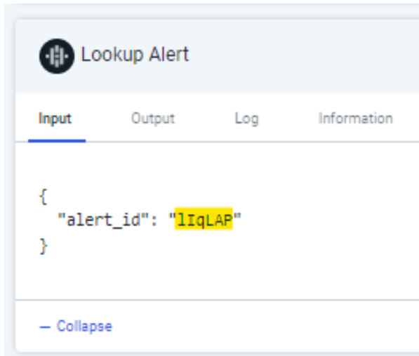
Figure 7. Input query sent to the Recorded Future API from InsightConnect. Note the only information needed is the alert identification code.
