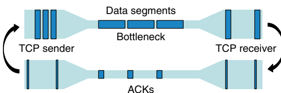
Figure 10.2 Self-clocking mechanism of the TCP connection.
