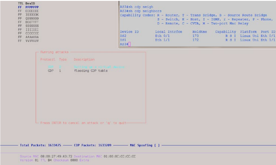
Figure 16-55. With CDP and LLDP disabled the DoS attack doesn't succeed
