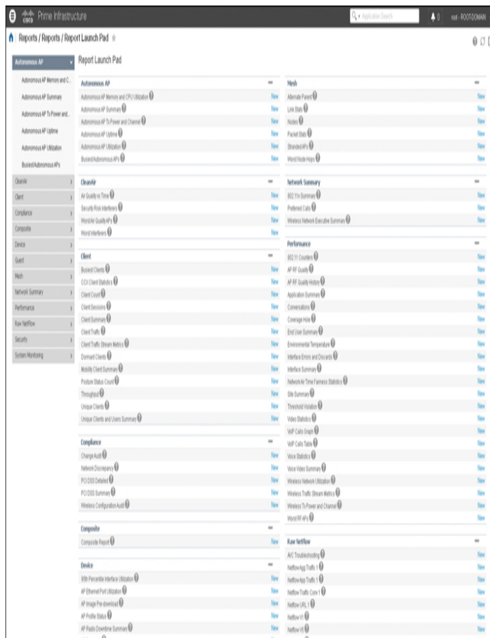
Figure 16-1 Cisco Prime Infrastructure Report Launch Pad (Upper Part)
