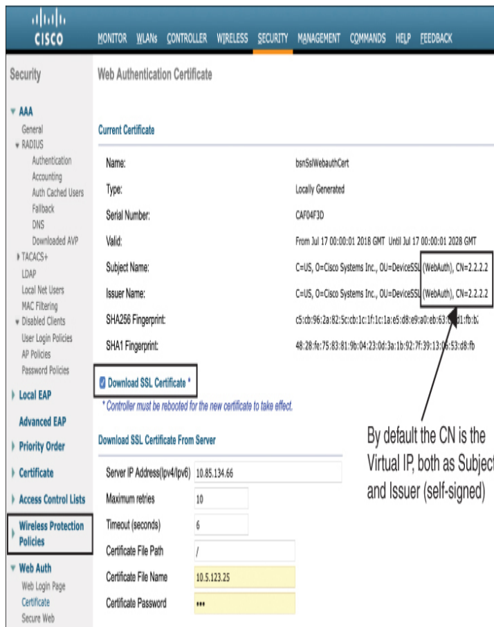
Figure 15-25 Web Authentication Certificates in AireOS
