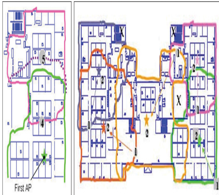
Figure 3-4 The Site Survey Process—Positioning More APs
