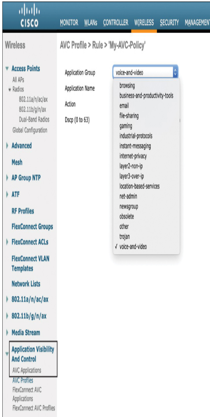
Figure 11-27 AVC Application Groupings in a New Rule
