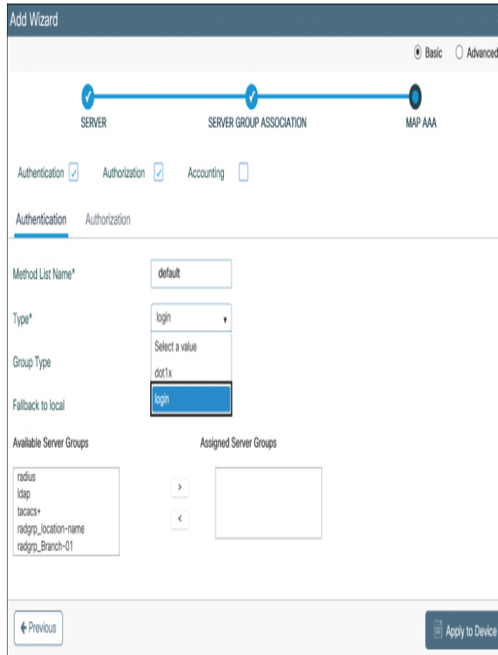
Figure 17-4 Configuring the Controller to Use a RADIUS Server for Management (Login) Authentication
