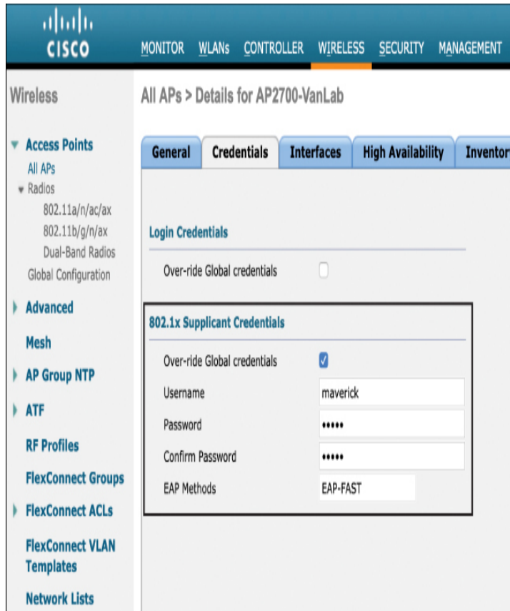
Figure 17-12 Configuring the AP with 802.1X Supplicant Credentials
