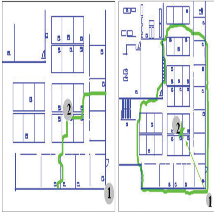
Figure 3-3 The Site Survey Process—Positioning the First AP
