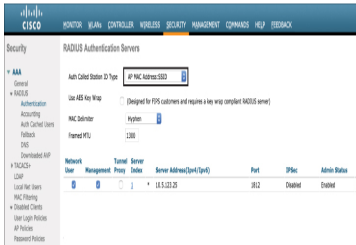
Figure 15-4 Setting the Auth Called Station ID Type
