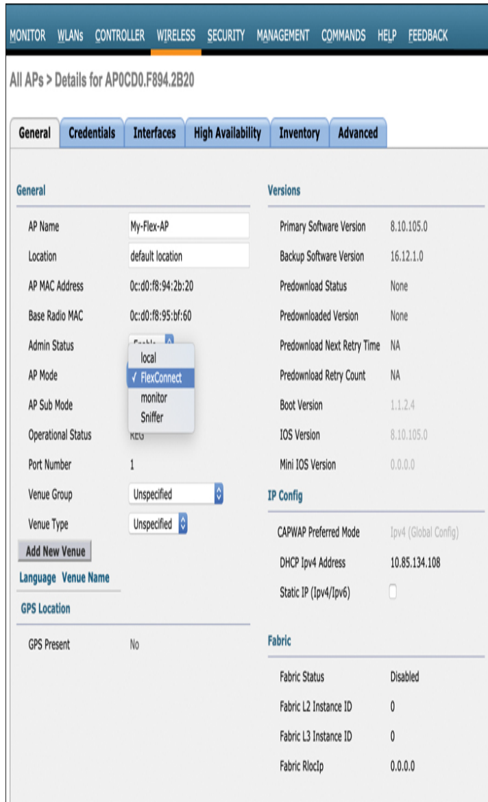
Figure 10-2 Changing the AP to FlexConnect Mode
