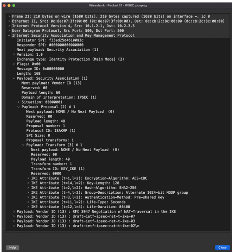
Figure 5-28. Wireshark capture of first Phase 1 packet
