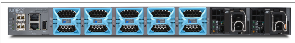
Figure 1-14. The rear of the Juniper QFX5100-24Q, illustrating the AFI airflow on the fans and power supplies
