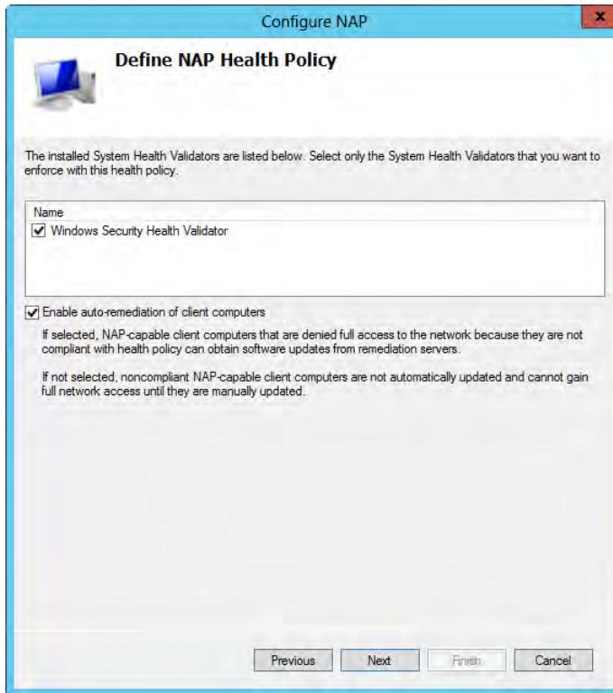
FIGURE 3-23 Configuring the SHVs to apply for this policy.
