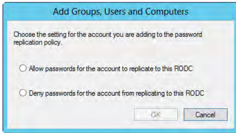
FIGURE 5-7 Adding a security principal to the Password Replication Policy.
