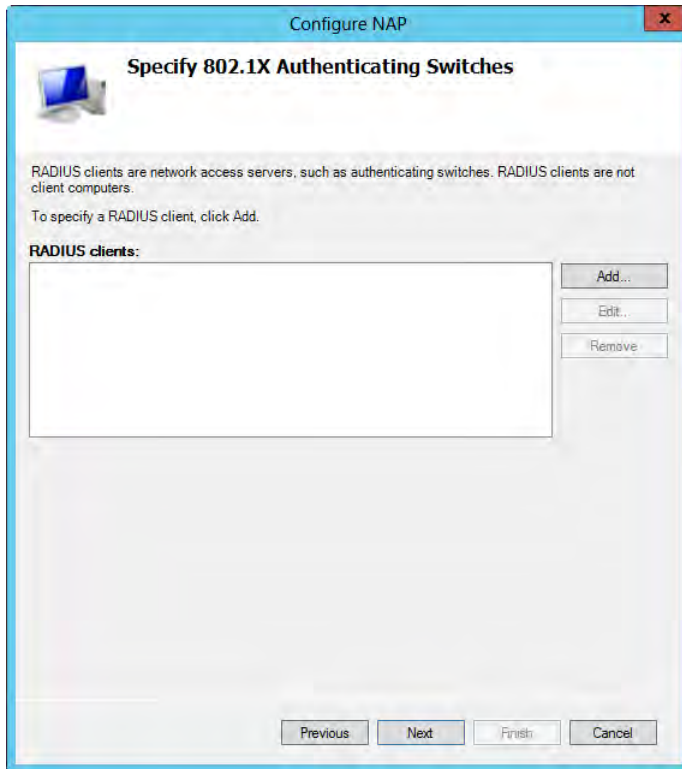
FIGURE 3-24 Specifying 802.1X switches for a wired deployment.
