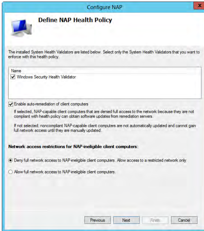
FIGURE 3-29 Defining the SHVs to be applied to this policy along with how to handle computers that aren't NAP-capable.
