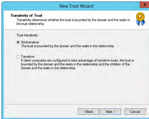
FIGURE 4-4 Setting the transitivity of the trust.
