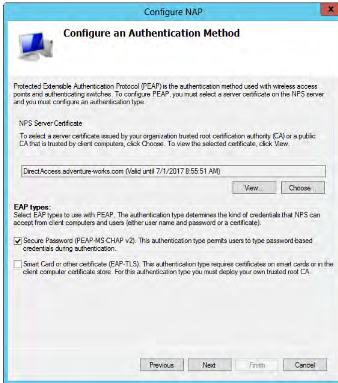
FIGURE 3-27 Configuring an authentication method as part of an 802.1X deployment.
