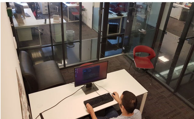
Fig. 1: Sensitive data is exfiltrated from the computer, modulated within the screen brightness, invisible and unbeknownst to the user. The video stream is recorded by a local security camera.
