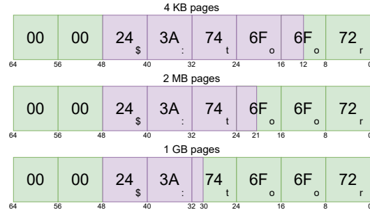
Figure 7: Depending on the page size, a number of virtual address bits (purple) can be retrieved via the TLB.
