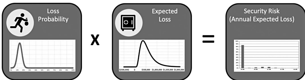
FIGURE 9.24 Quantitative security risk analysis through Monte Carlo Simulation. When the values of the security risk equation variables (loss probability and expected loss) are represented by pdfs (or probability mass functions), computing the ALE to a security risk such as ransomware can be performed through Monte Carlo simulations.
