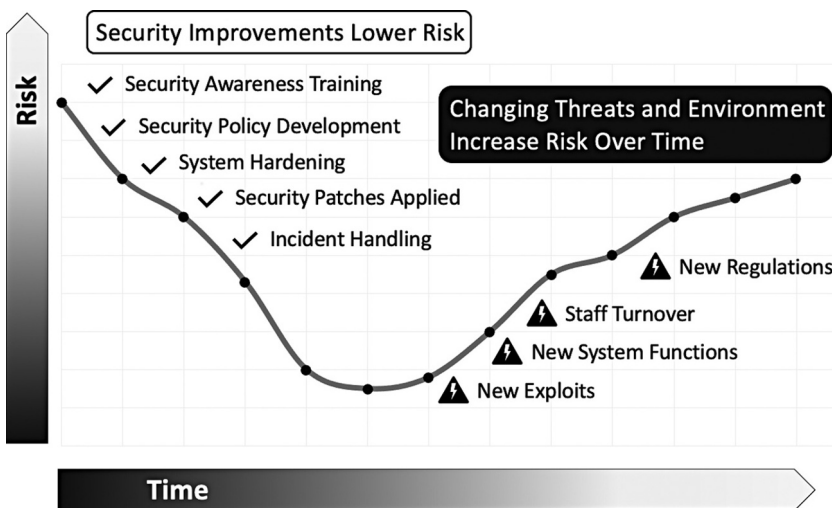
FIGURE 1.3 The eroding security posture. Applying security improvements such as security awareness training and security patching can lower the security risk of an information system, but the changing threats and environment will erode the security posture over time.
