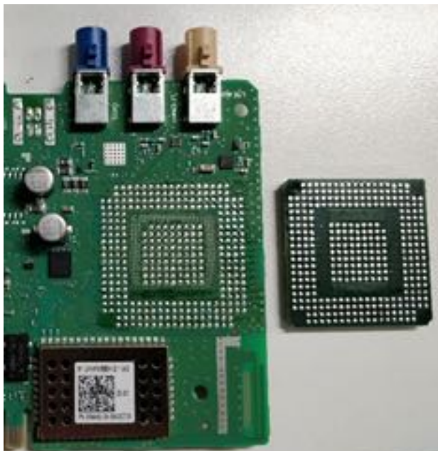
Figure: The LGA paddings of LTE module
