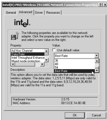
Figure 6-17: Configuring the data rate of the client radio
