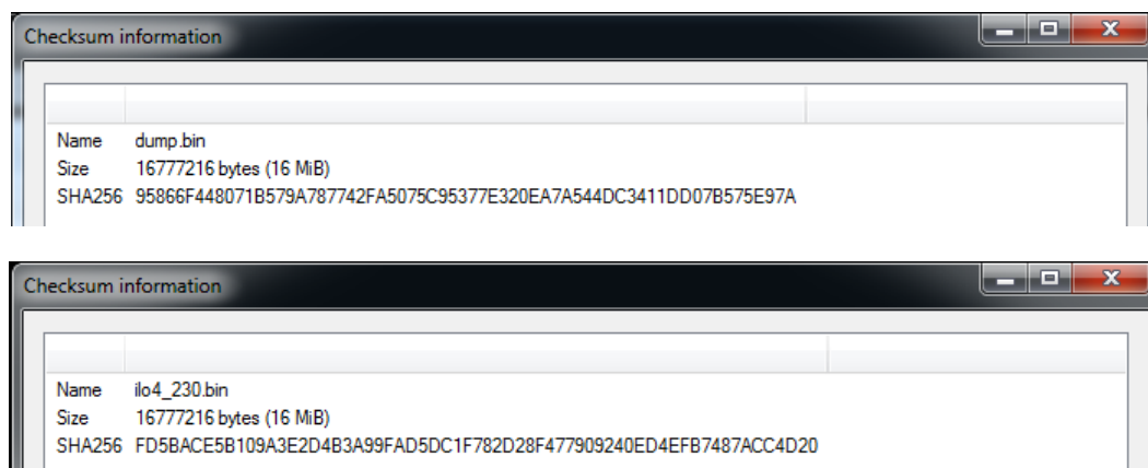
Figure 6 - Firmware Signature Difference: (Top) Infected dump obtained; (Bottom) Original version provided by the HP Company
