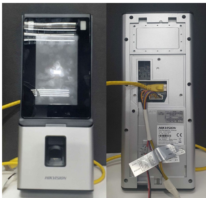
Figure 9. The front and back of the Hikvision access control device
