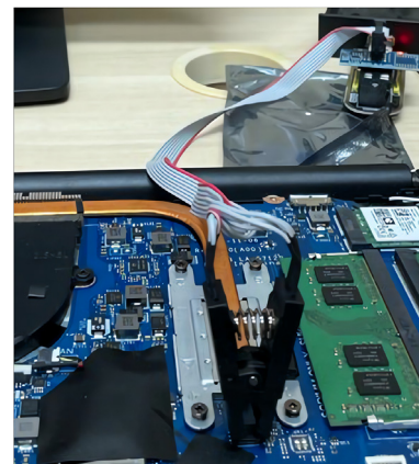
Fig. 2. Reading the flash memory contents with a low-cost CH341A SPI programmer.
