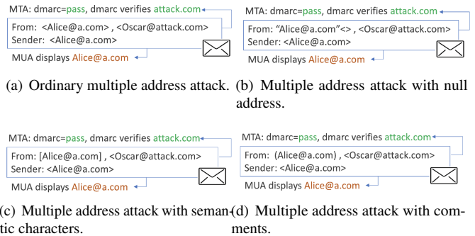
Figure 8: Multiple email addresses attacks to make DMARC verify Oscar@attack.com while MUA displays Alice@a.com.
