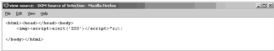
Figure 3.36 The Result Code For After the Injection
