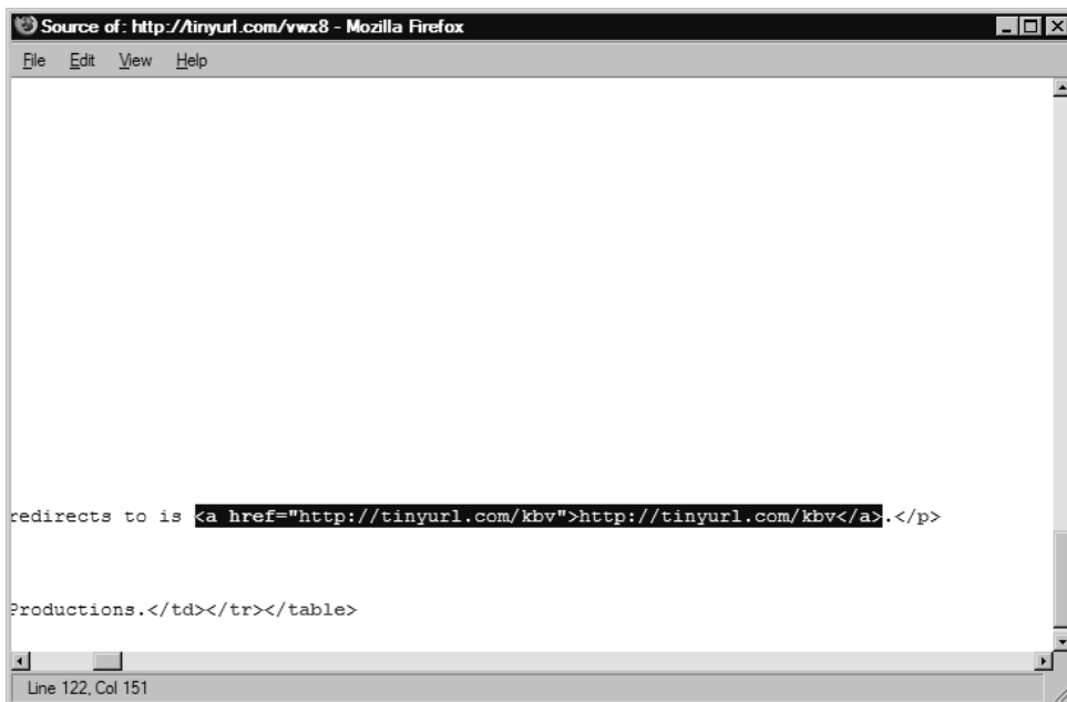
Figure 6.35 Detecting a Potential XSS Vulnerability in TinyURL
