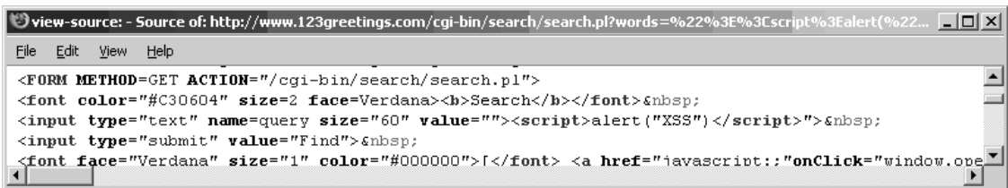
Figure 3.33 View Source of the Necessary XSS Payload
