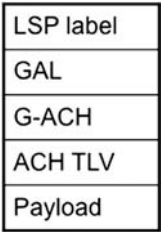
Figure 17.4 Packet headers for OAM packets in MPLS-TP
