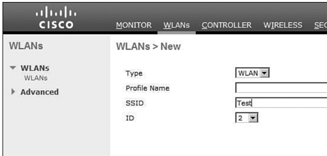
Figure 16-2 Cisco Wireless Controller Configuration Screen for Setting the SSID
