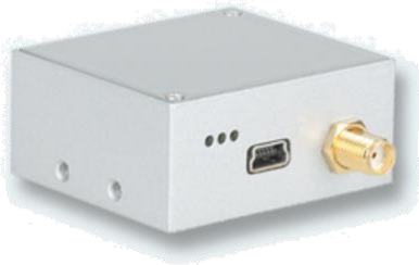
Figure 33. GSM-R Triorail TRM-5T modem
