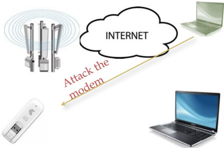
Figure 34. A Bad USB attack using a modem
