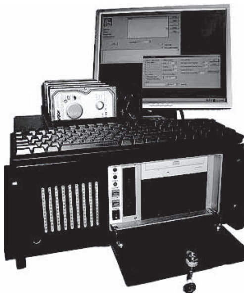
Figure 2-11 The ImageMAStter 6007SAS performs high-speed data duplication over local or network connections.
