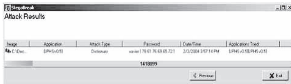
Figure 1-34 StegoBreak allows the user to obtain a password used for steganography.
