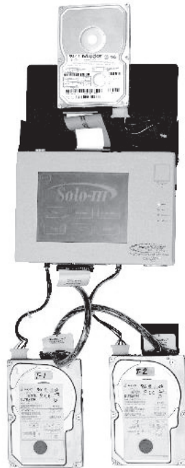
Figure 2-4 The Image MASter Solo-3 performs high-speed data acquisition.
