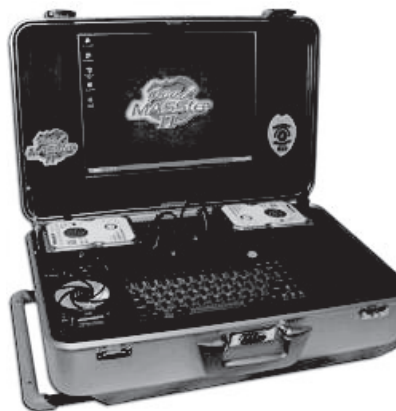
Figure 2-6 The RoadMASter-2 is used for data acquisition in the field.
