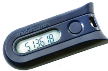
FIGURE 4.2 Hardware-based multifactor authentication token
