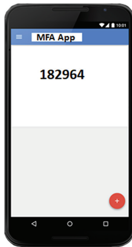
FIGURE 4.3 Smartphone-based multifactor authentication token
