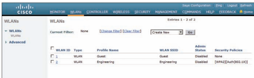
Figure 15-15 Displaying WLANs Configured on a Controller
