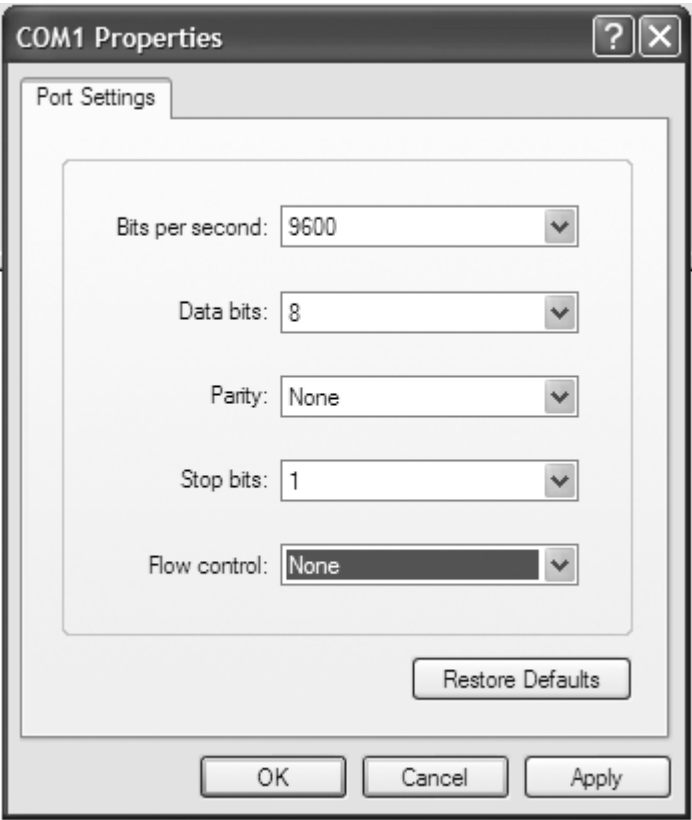
Figure 4-5 PC Settings to Connect to a Router or Switch
