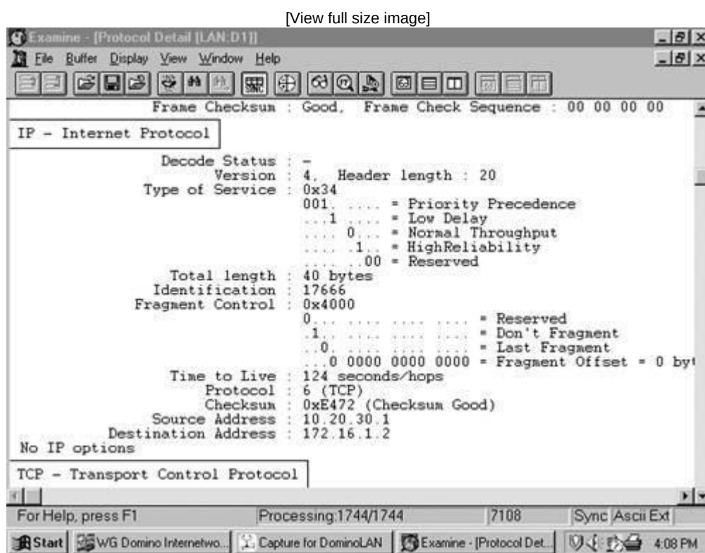
Figure 14-7. Pogo's policy route has set the Precedence bits of this packet to priority (001b) and the TOS bits to minimum delay and maximum reliability (1010b).
