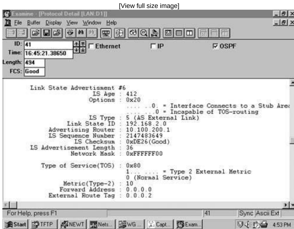
Figure 14-11. This type 5 LSA is advertising network 192.168.2.0, which is in domain 2, within the OSPF domain. The route tag is shown on the last line.
