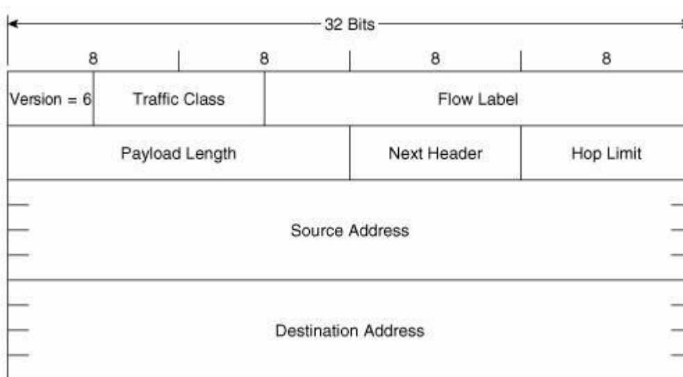
Figure 2-5. The IPv6 packet header.
